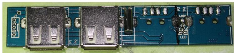
3. Cut the PCB on the black line between the two de-soldered USB connector;
